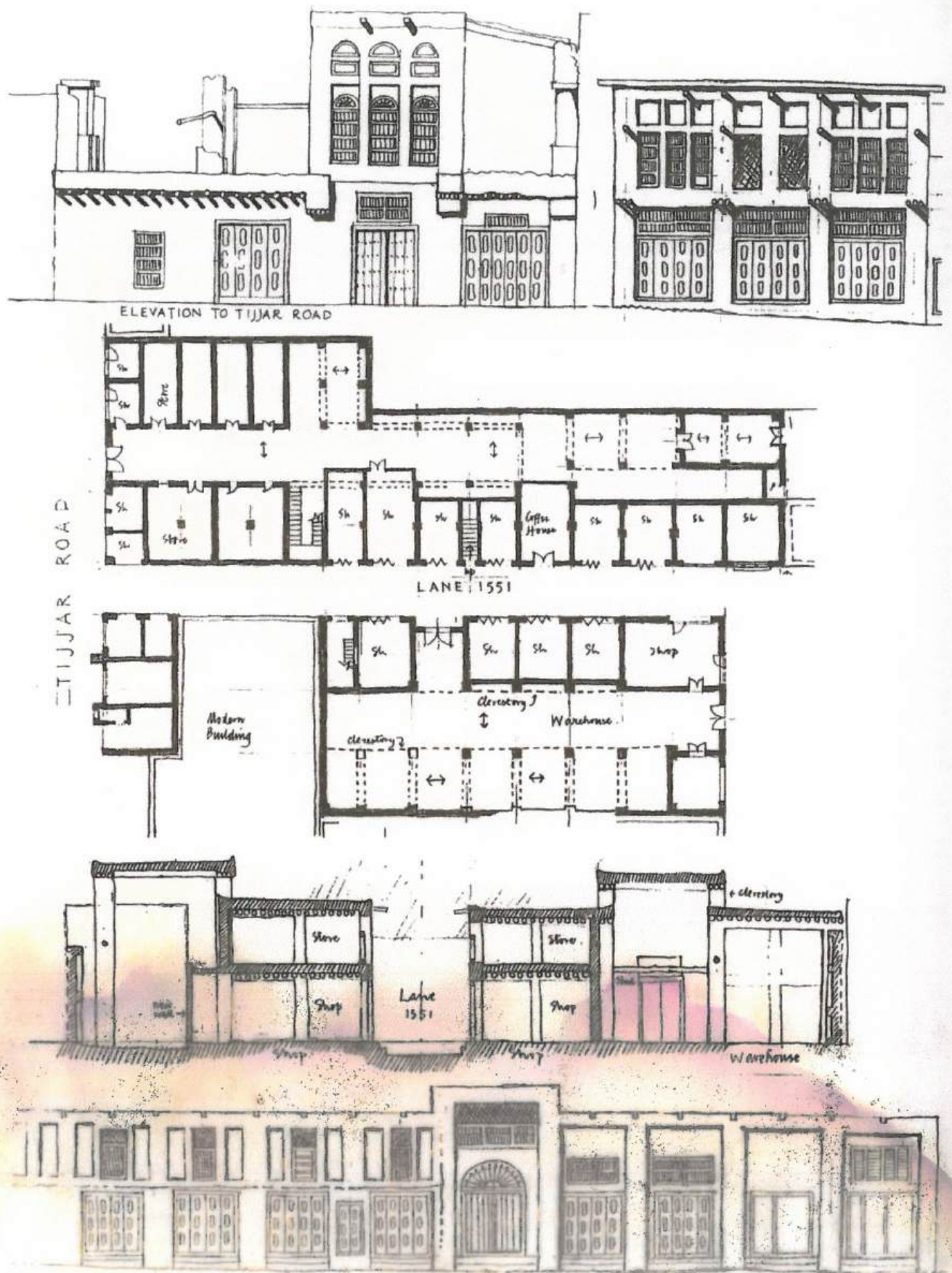
Fig 5.6 (top left) Amara and Khan on Tijjar road. Fig 5.7 (top right). Workshops and Khan on road 1339. Fig 5.8 (bottom) Amara and shops on lane 1551 and Tijjar road; plan, section and elevation to lane 1551.
