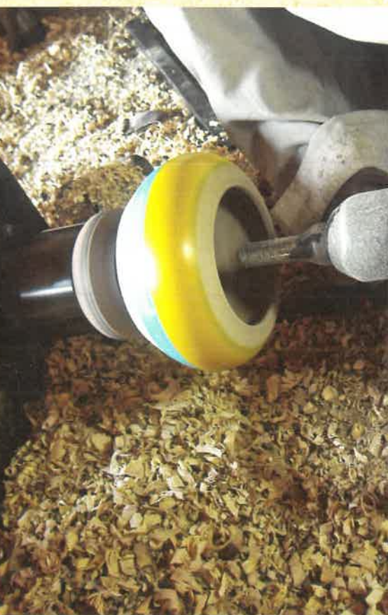
Sillanwali – Workshop of Muhammad Hanif. An 'abri' (cloud) design is being created on the outer surface of a powder box. The entire process is completed on a lathe machine.
