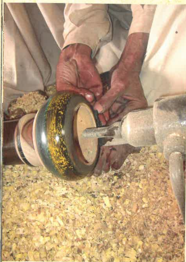
Sillanwali – A powder box is being prepared on a lathe machine.
