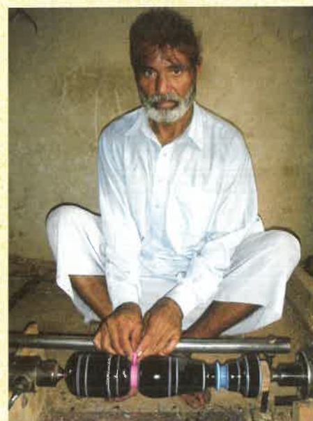
Mid Ranjha – Lakh colour is being applied on a 'paya' while still on lathe by Muhammad Ashraf alias Maulu.
