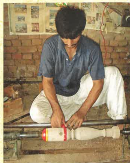
Mid Ranjha – A paya is being wrought on a lathe.
