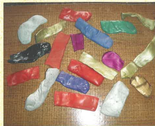
Sillanwali – Color sticks called 'battis' of lakh for applying color on wood while still on lathe machine.
