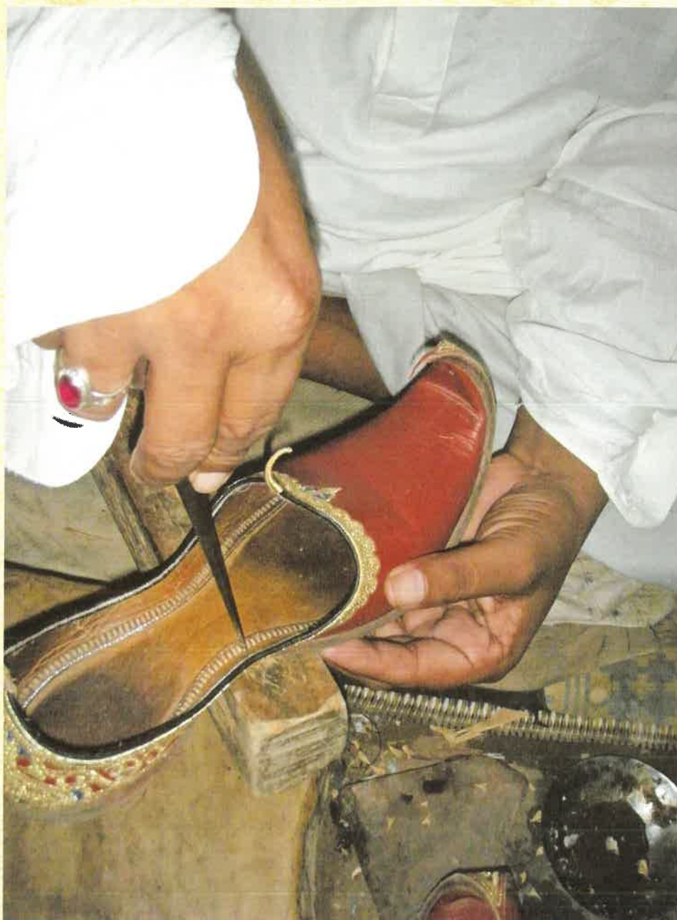
Kot Momin – A sole is being joined with the 'upper' of a desi-jali.
