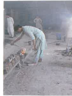
Smelting to produce toilet fittings.
