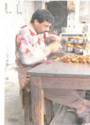
Motor winding for fans.
