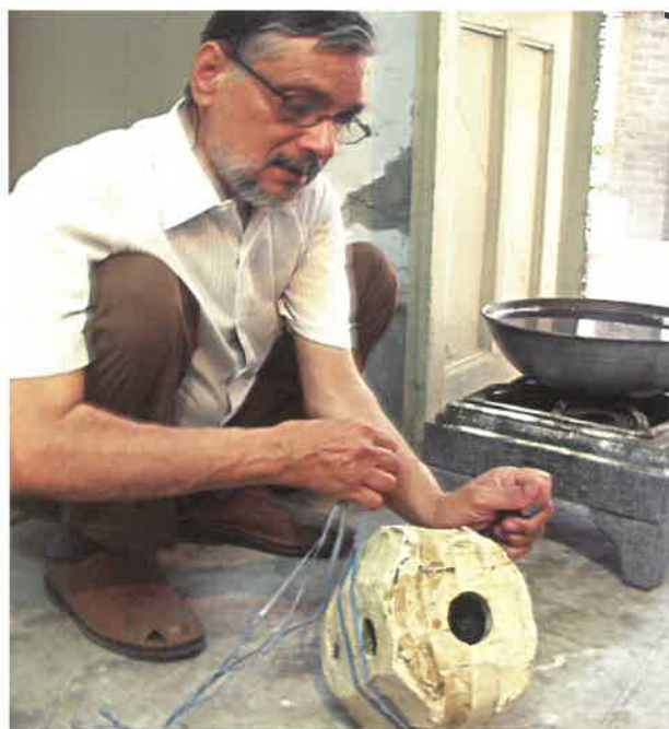
Fig. 11 - Tighten the two pieces firmly with rope
