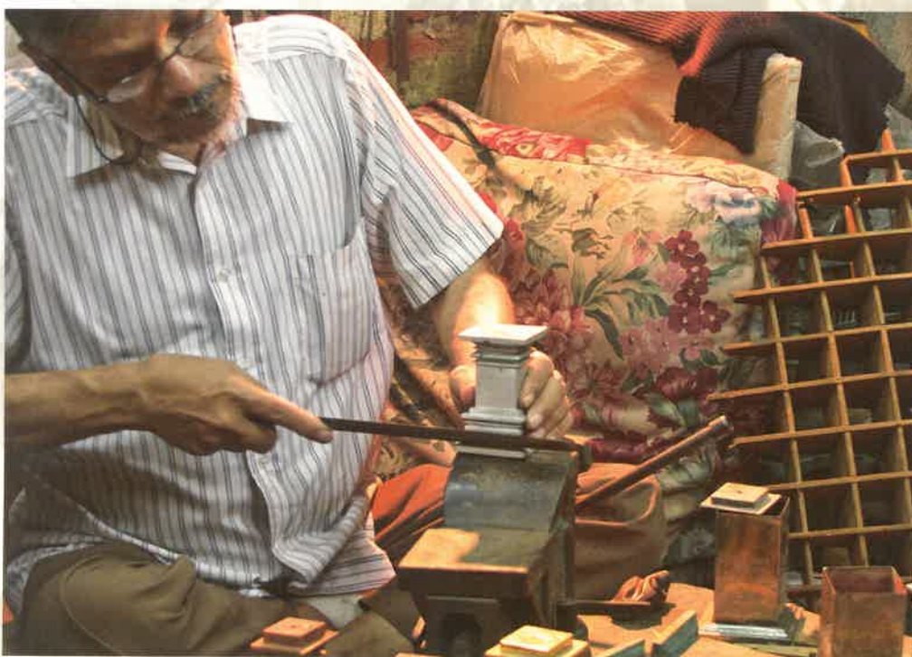
Fig. 5 - Fig. 6 - Above: fixing the sculpture on the pedestal. Below: filing the base of sculpture.
