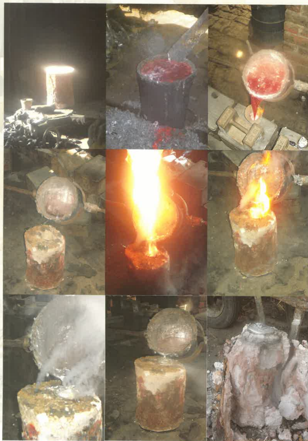
Fig. 36. Metal Casting Process – melting the metal, metal pouring and separating lost wax metal piece from the refractory mould.
