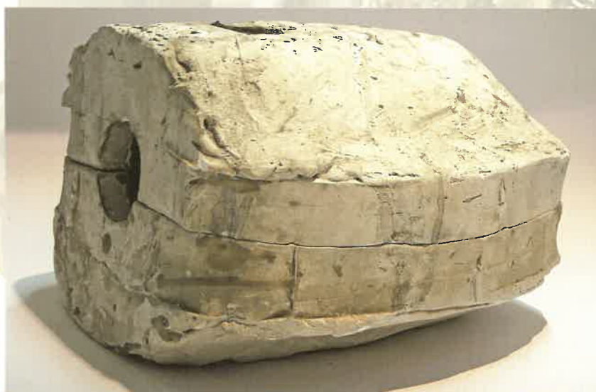
Fig. 3 - Rubber mold and jacket with sculpture in the center separated by clay, PVC is poured from upper hole. Invert jacket for other half PVC filling.
