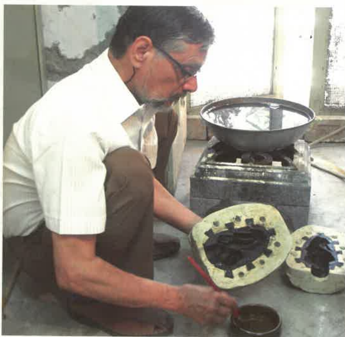
Fig. 9 - Open the mold and apply liquid Alum on both the parts of PVC rubber mold
