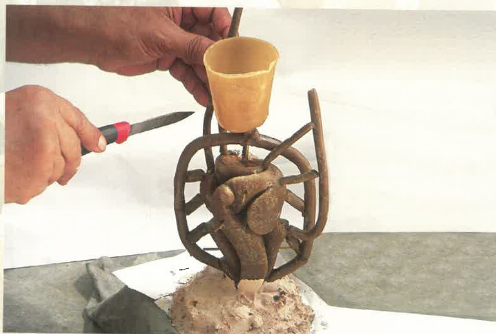
Fig. 29 - Fix the pouring cup with wax rods
