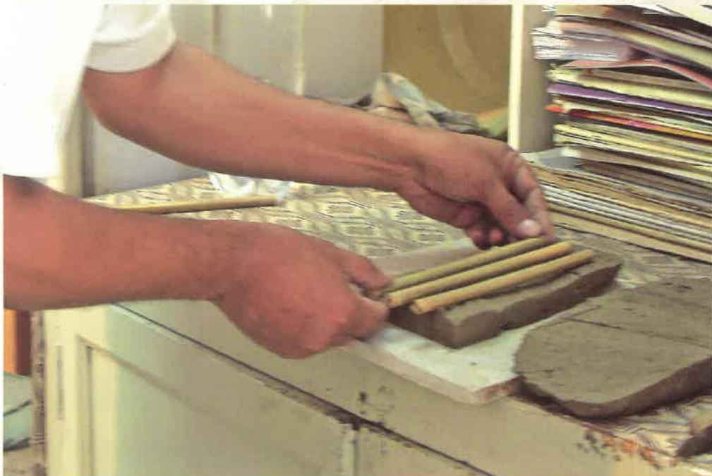
Fig. 24 - Clay mold for making wax bars using reed sticks
