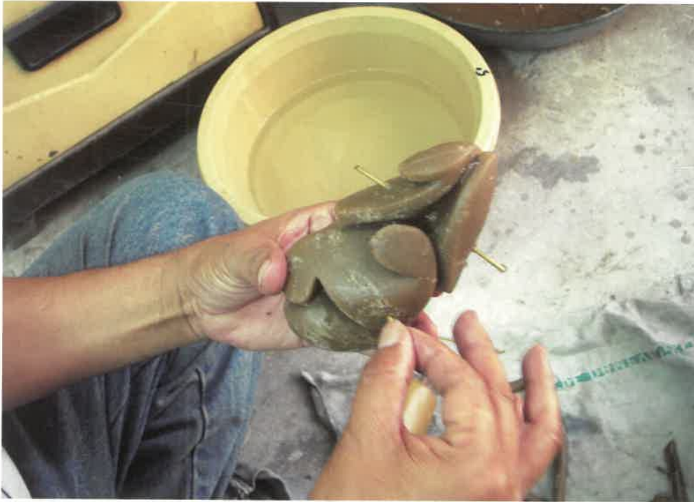
Fig. 19 - Insert three to four nails/pins across the wax sculpture
