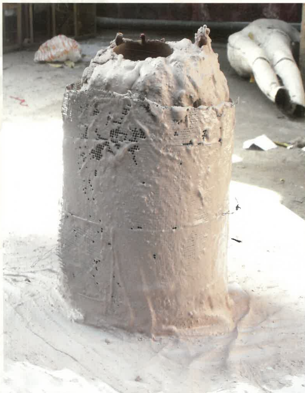
Fig. 33 - Apply more refractory to strengthen the mold and leave it to dry for 3 to 4 days. When dry, remove wax by placing in heated kiln and then pour molten metal of choice into the mold to obtain the final thin-metal hollow light-weight casting. This entire process is called as Hollow Casting or Lost-Wax Casting.
