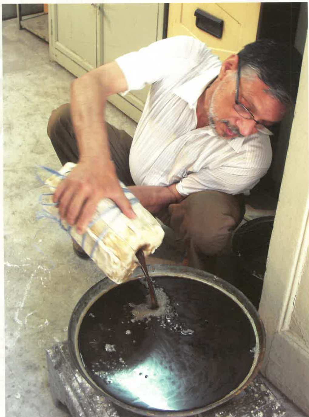
Fig. 13 - After achieving sufficient thickness of the wax cast, drain off excess wax. Remember that the wax core has to remain hollow and the cast walls thin enough for the desired result
