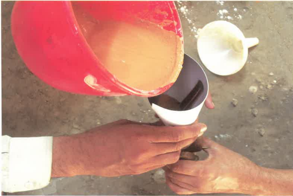
Fig. 23 - Now pour the prepared refractory mixture into the core after placing wax string in center of the core
