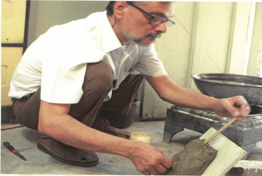
Fig. 25 - Remove reed sticks from clay to obtain mold for pouring wax
