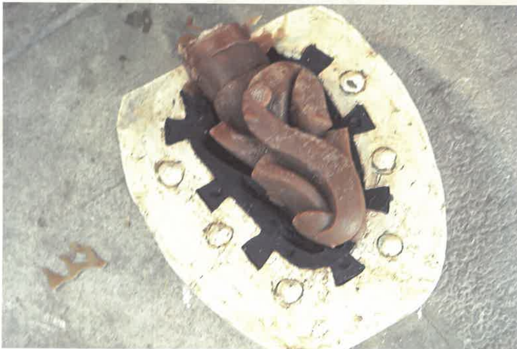
Fig. 15 - Remove one side of the mold
