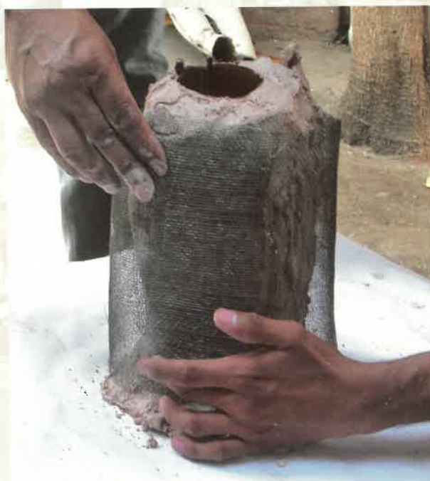
Fig. 32 - Fix the Mesh around and cover all sides with refractory materials to strengthen mold for pouring the metal.
