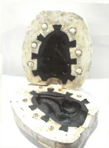
Fig. 4 - Two pieces of rubber mold with jacket. Notice the dovetail keys for alignment.
