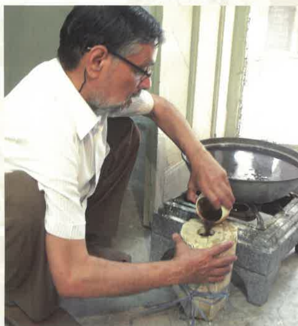
Fig. 12 - Pour wax 2 or 3 times in the rubber mold. Shake & rotate the mold to cover inner walls of the PVC mold with wax of desired thickness.
