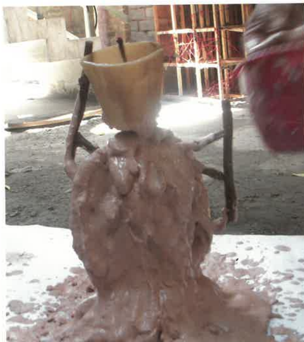
Fig. 31 - Cover all the sides with refractory mixture
