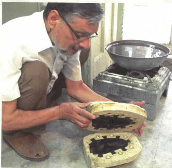
Fig. 10 - Put both sides of the mold together
