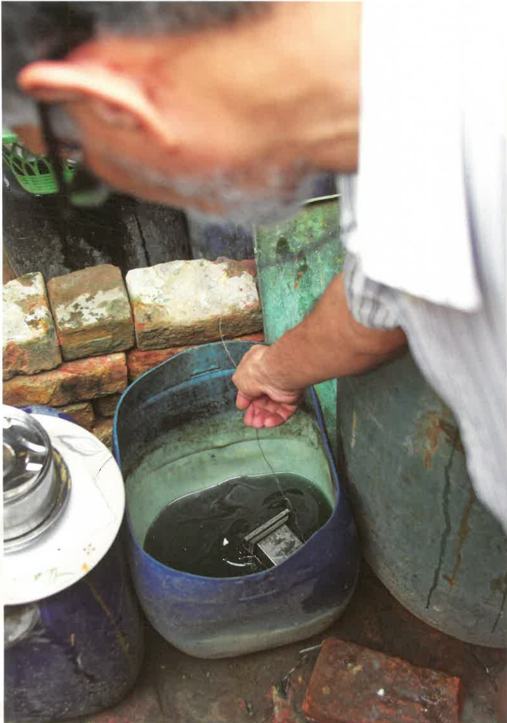
Fig. 17 - After soldering the object it is placed in a strong acid for 3 to 5 minutes to remove the chemical to make it ready for polishing.
