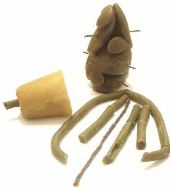
Fig. 27 - Pouring cup of wax for runner, the riser, wax string and wax bars
