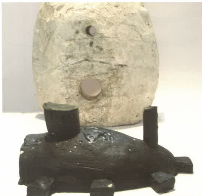
Fig. 7 - PVC mold and plaster of Paris jacket
