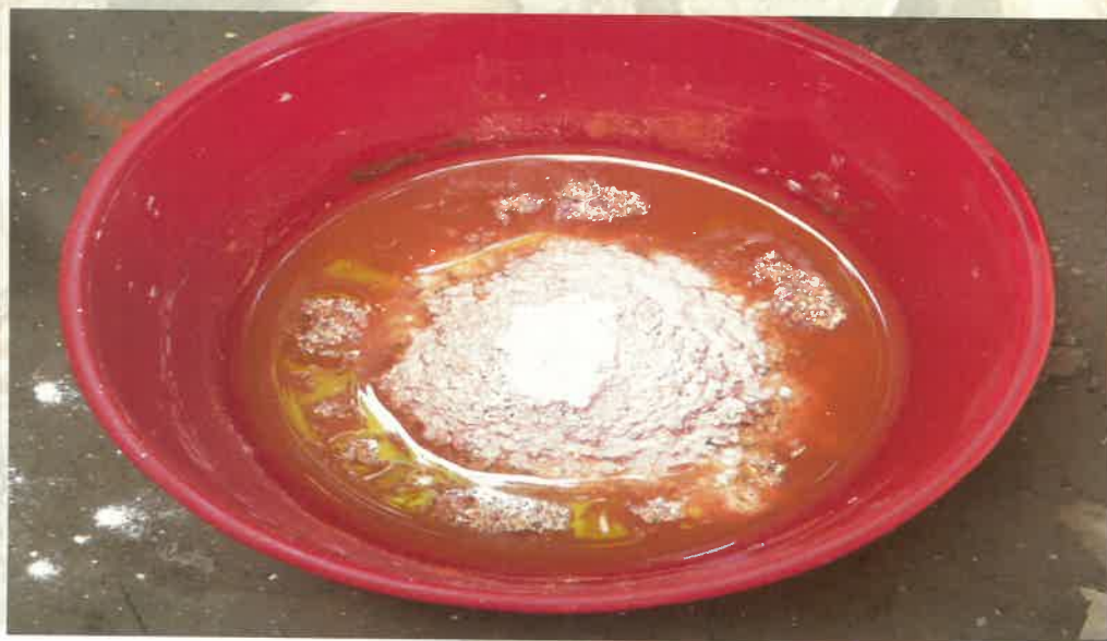
Fig. 22 - Make refractory mixture with three components in water with ratio 1 part grog, 1 part brick dust & 2 parts plaster of Paris to achieve consistency of yogurt
