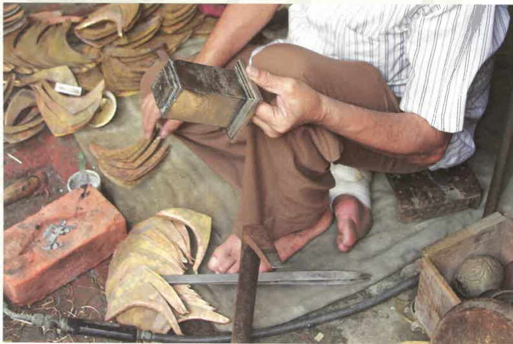
Fig. 15 - Fig. 16 - Above : Soldering the pedestal of sculpture. Below: Finishing the base of sculpture.
