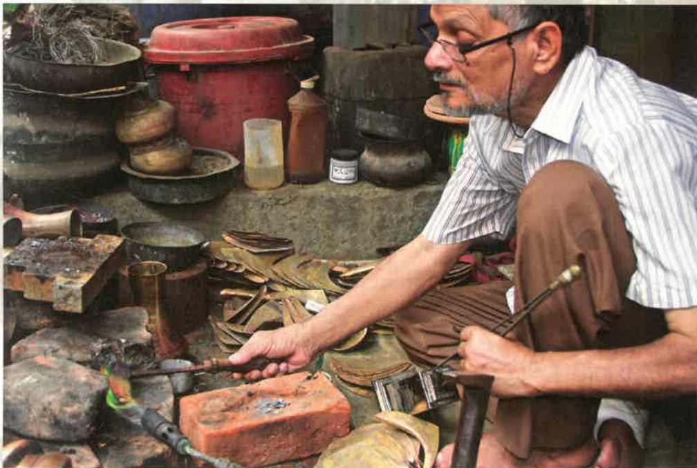
Fig. 13 - Fig. 14 - Above: Soldering the pedestal. Below: Heating the soldering iron called Cavia in local language.
