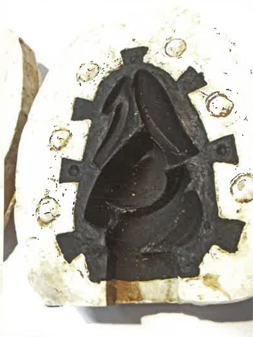
Fig. 5 - One piece of mold casted in PVC rubber. Notice the marble spots in PVC leys for PVC mold alignment.
