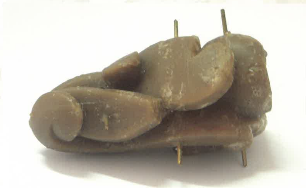
Fig. 20 - Inserted nails through the wax sculpture now ready to fill the core
