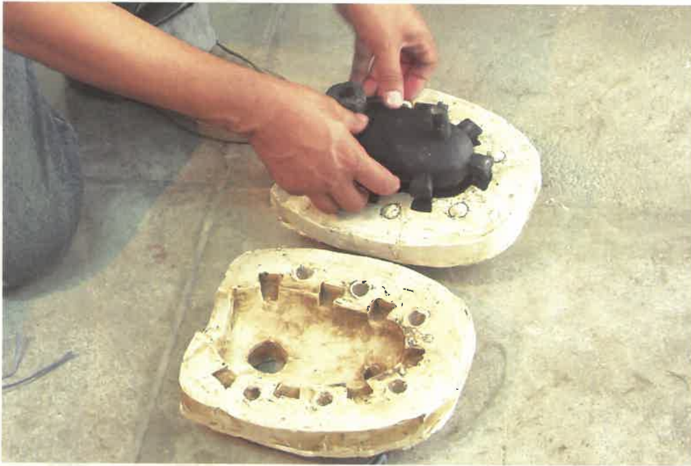
Fig. 16 - Remove the second side of the mold
