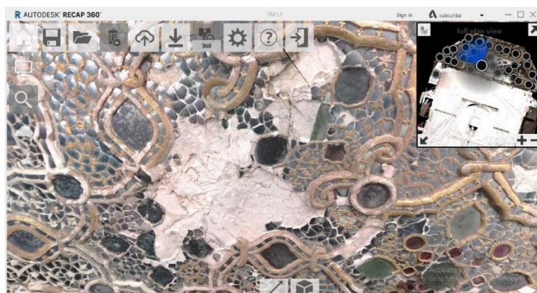
Figure 5-38: RGB 3D Model of Ornamentation in Autodesk Recap 360 Pro
