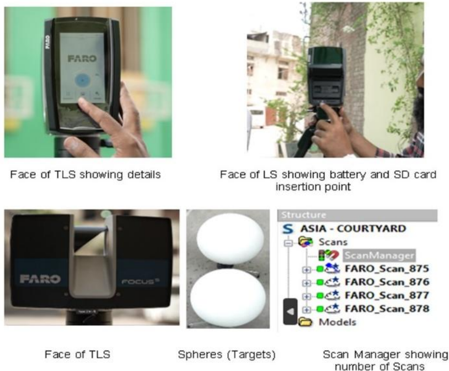
Figure 7-3: Faro Focus S (TLS) Spheres (Targets) and Scans surveyed at the site
