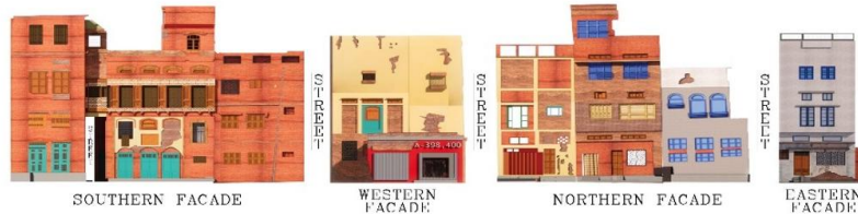
Rendered Elevations of Buildings around Choara Khoo with 3D Faro Laser Terrestrial Scanner (By WCLAI in 2016)
