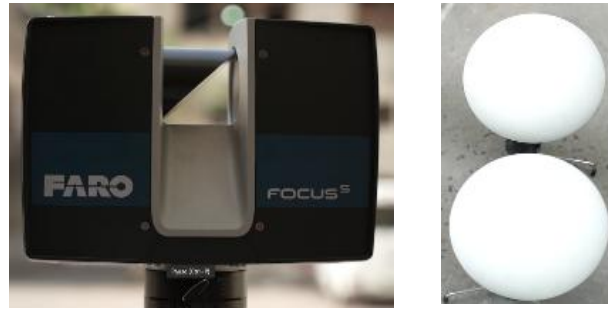
Figure 5-33: Faro Focus S (TLS) (Left) and Spheres (Targets) (Right)
