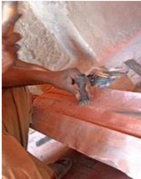
Figure 124: Carver is removing the Chunks with the help of Hammer and Tooth Chisel.
