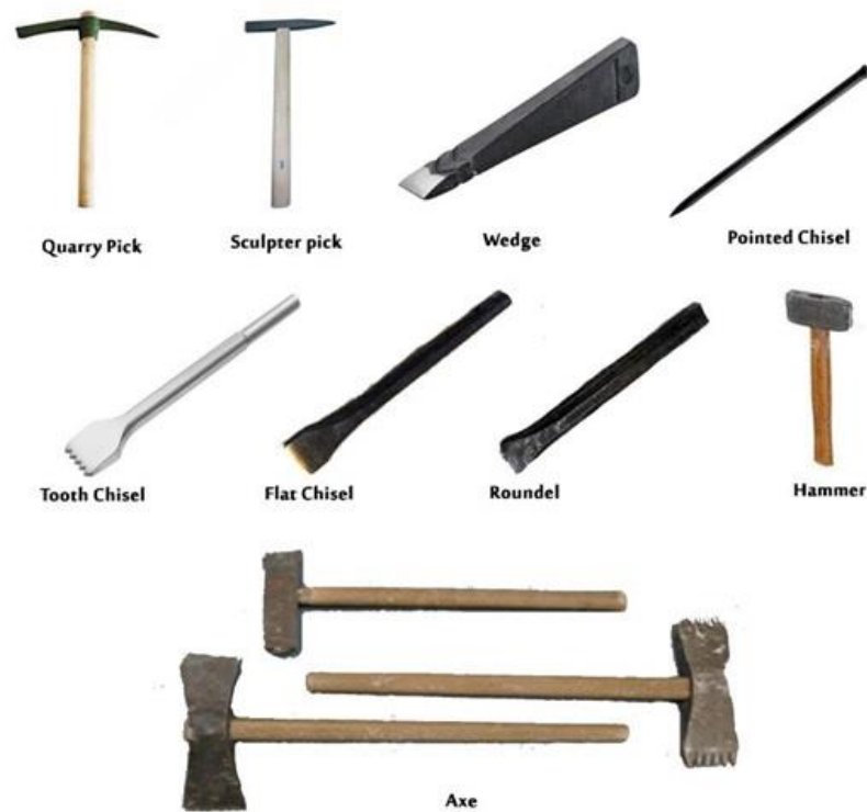
Figure 125: A Set of Modern Tools are used in Latticework.
