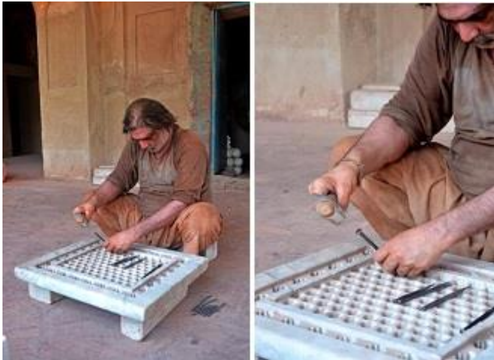
Figure 118: A Carver using a Chisel and a hammer to shape a stone.
